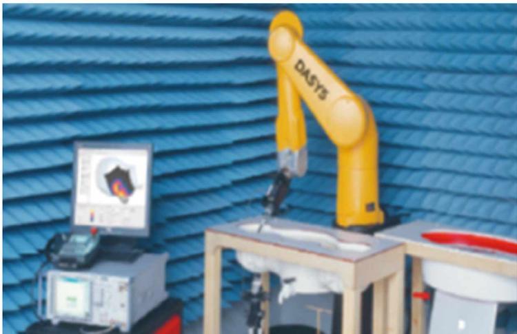
**FIGURE 2** Robotic arm with electric field probe. Source: Speag DASY 52 Info Sheet.
