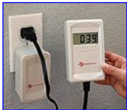
GS Filter to reduce dirty electricity between the range of 4 to 100 kHz
